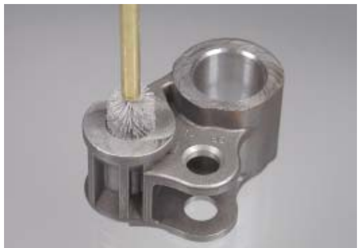
Stahlgußschwinge, Entgraten von Bohrungen Cast steel oscillating crank, Deburring the drill holes
