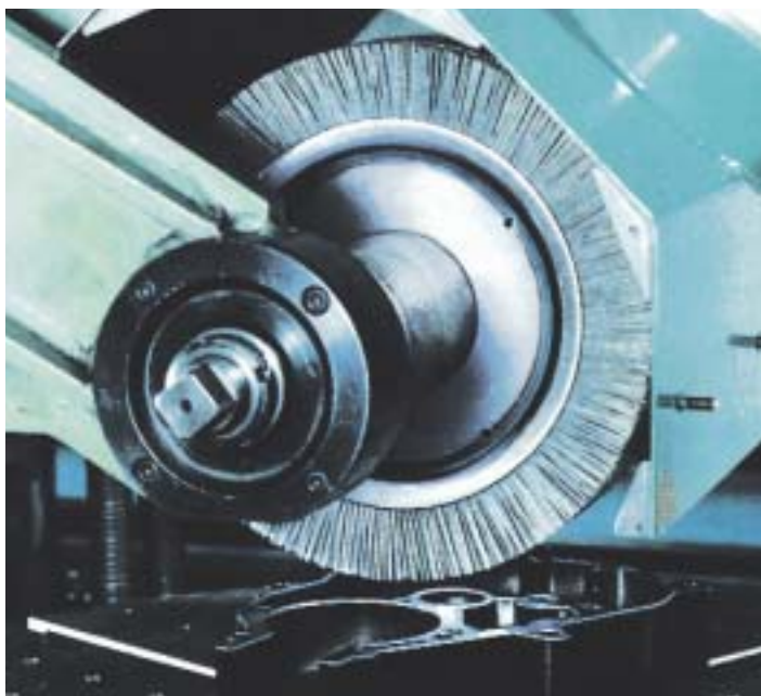
Entgraten von Aluminiumprofilen. Deburring of aluminium profiles.
